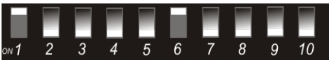
DIP switch setting for audio disabled with timed relay active, alarm zone 1, radio channel 0
